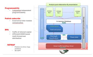
On top of this framework is possible to build any analysis application, called *analyzer App*, that can elaborate traffic information extracted by DATI at its own convenience. An *analyzer App* can be written in any language whith the only requirement to have a **REDIS** library to interface with the in-memory database and pub/sub facility.
