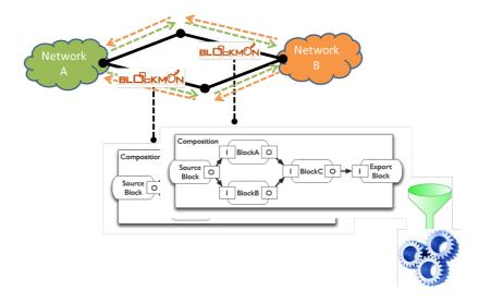
Blockmon is based around the notion of *blocks*, which are small units of processing (e.g., packet counting). Blocks are connected and communicate between each other via gates. Among other functionalities, Blockmon provides an implementation of Tstat passive probe as result of collaboration activities within the mPlane project.
