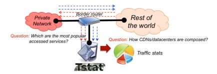
As shown in the figure, Tstat can produce real time analysis processing live traffic acquired from both standard PC NICs (using the libpcap) or DAG cards. Moreover, it can also process previously recorded packet-level traces of various formats (libpcap, snoop, etherpeek, etc.).
