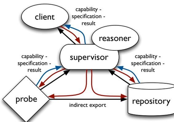
**Figure 1: The mPlane Architecture**
